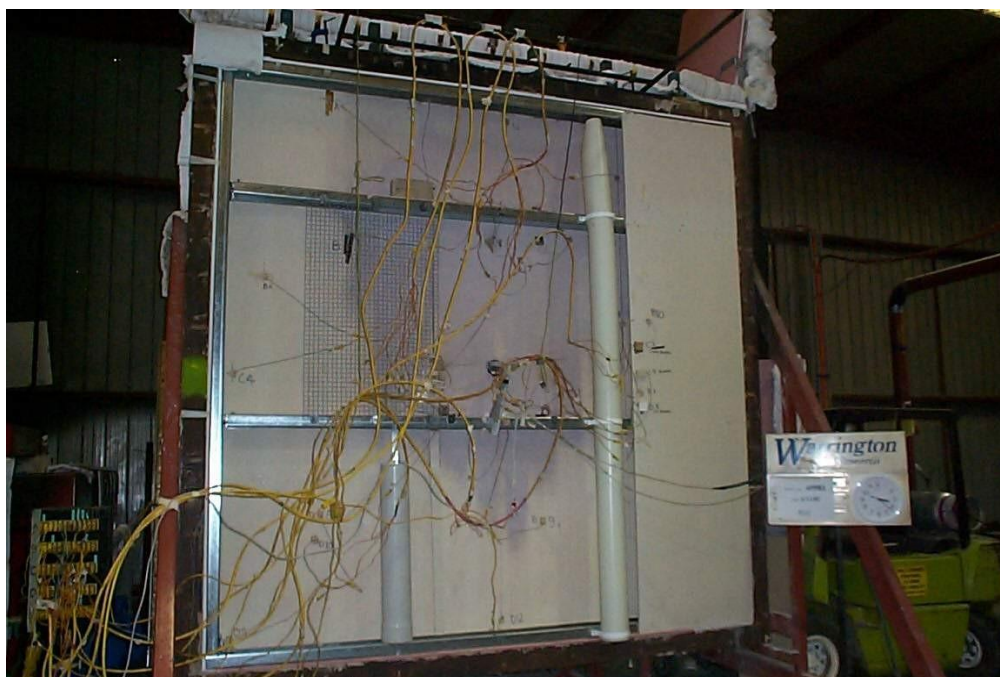
Figure 4 Unexposed side of wall system
